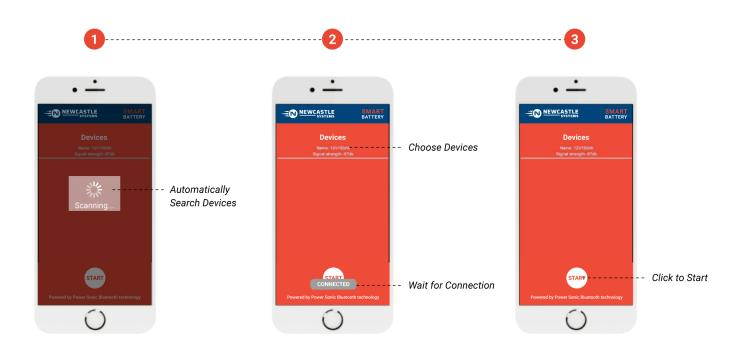
If you have selected a battery to connect with and the app is not confirming the connection, it may be because someone else has already connected to the battery. Only one device can be connected to a battery at any one time.
