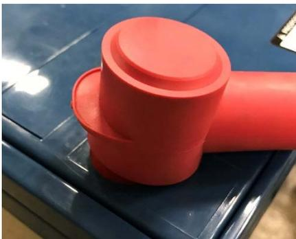
**5.** Pull rubber boot over tightened terminal.
