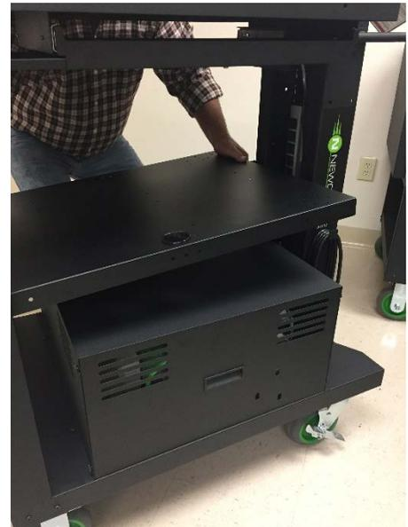
**1.** If second shelf was purchased, remove it to gain access to battery box (Allen wrench required).
