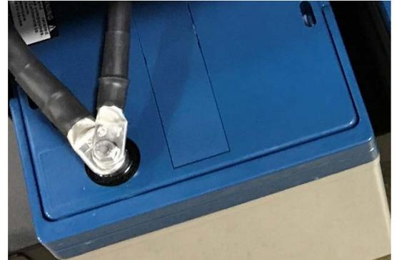
**6. Negative Connection, Battery 1:** Take bolt and place flat washer, black connector wire (D1) and large black wire (C) onto bolt (as shown above); insert into negative (-) battery terminal.
