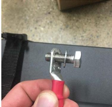
**3. Positive Connection, Battery 1:** Take bolt and place flat washer and large red wire (A) onto bolt (as shows above); insert bolt into positive (+) battery terminal.
