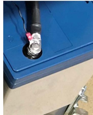
**9. Negative Connection, Battery 2:** Take bolt and place flat washer, small black wire (E), and black connector wire (D2) onto bolt (as shown above).
