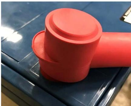
**5.** Pull rubber boot over tightened terminal.
