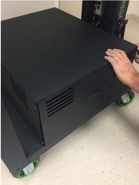
**3.** Remove front battery panel by loosening the thumb screws.
