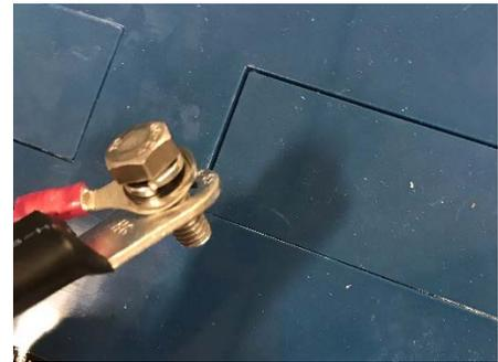
**6. Negative Connection:** Place lock washer onto bolt first, then flat washer, then small black wire (C), then large black wire (B) in order shown above.
