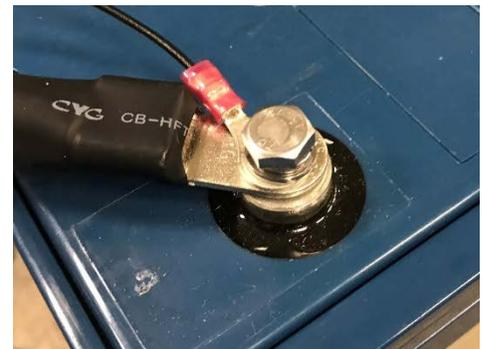
**7.** Securely tighten terminal bolts with a 10mm wrench.
