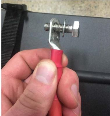
**7. Positive Connection, Battery 2:** Take bolt and place flat washer, large red wire (B) onto bolt (as shown above); insert bolt into positive (+) battery terminal.
